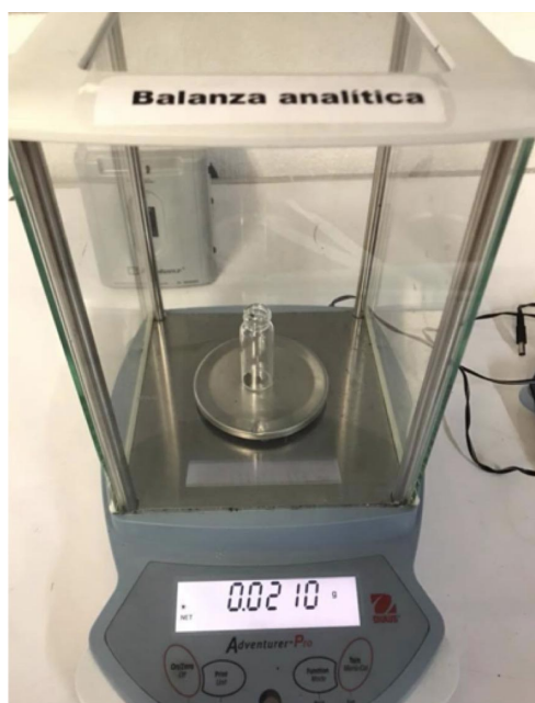
Fig. 1. Weight of the exact amount of Rhodamine B on the analytical balance (Adventure pro®).
