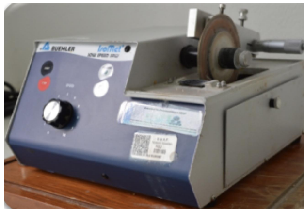
Fig. 2. Low speed Buehler IsoMed® trimmer.
