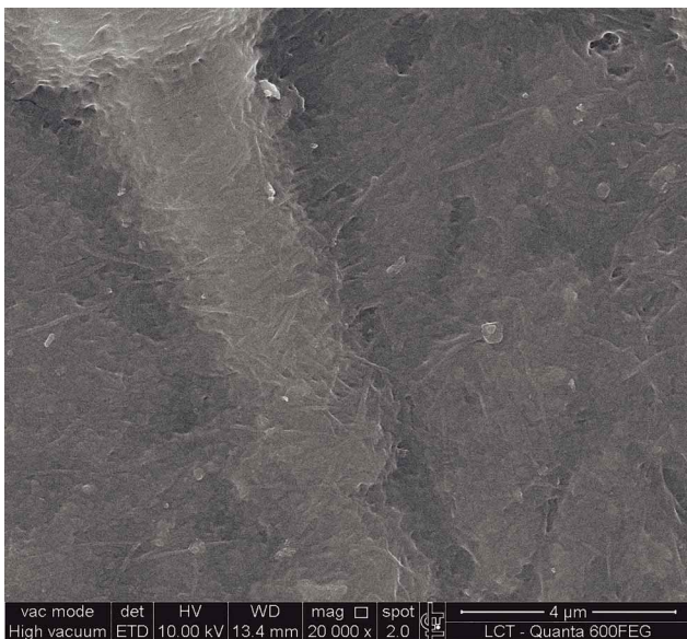
Fig. 4. A closer view of the areas, previously mentioned, showing a good sealing after 18 months.
