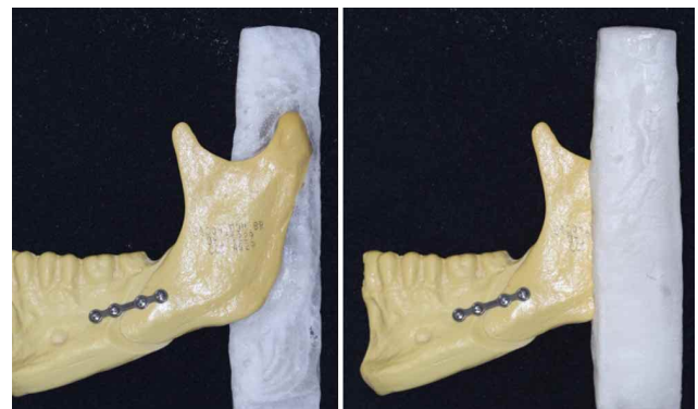
Fig. 7. Jaw inserted in acrylic resin base.
