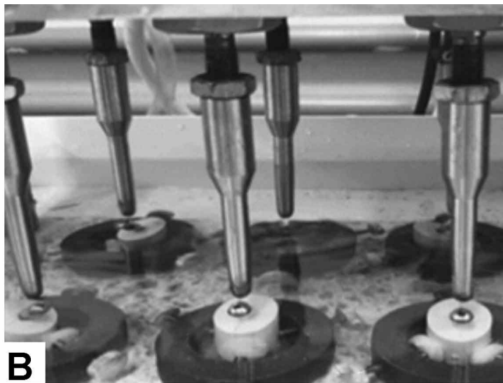
Fig. 2. Specimen used for mechanical fatigue aging tests. A) Sample with micro abutment and crown installed. B) Specimens placed in the fatigue testing machine.
