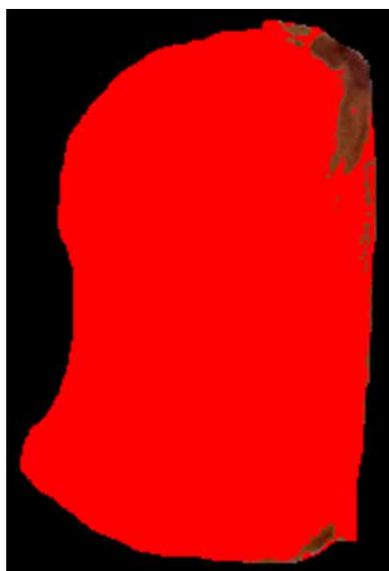
Fig. 1. Sample of Color Threshold Method used to calculate stained area.
