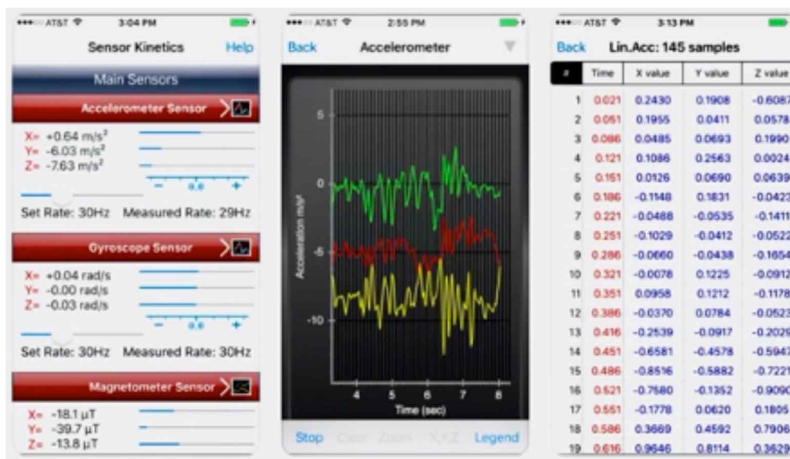
Fig. 6. Example of application showing the x, y, z axes: on the left, in the center, the accelerometer graphs, and numerical data on the right.
