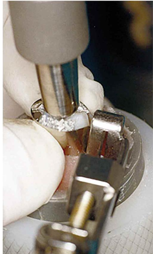
Fig. 3. Steel sphere in contact with dental restoration and cusps.
